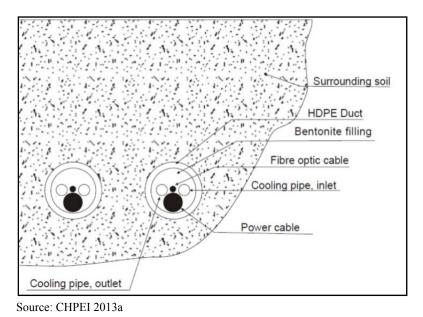
Figure 2-12. Representative Schematic of Cooling Pipes inside an HDPE Conduit
