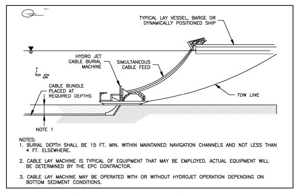
Figure 2-14. Typical Aquatic Transmission Cable Installation Process
